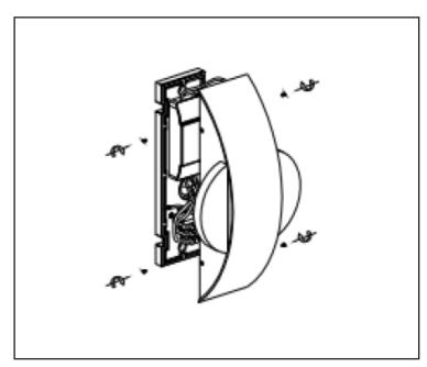
Attach the light fitting to the wall plate and insert the retaining screws to secure.
