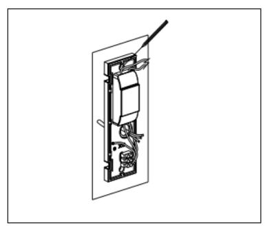
Mark out your drilling points using the wall plate as a template and pierce the cable entry hole making sure there are no jagged or sharp edges.
